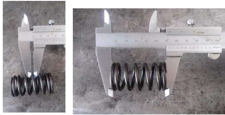
Fig. 4. Measurement of the cylinder head springs
