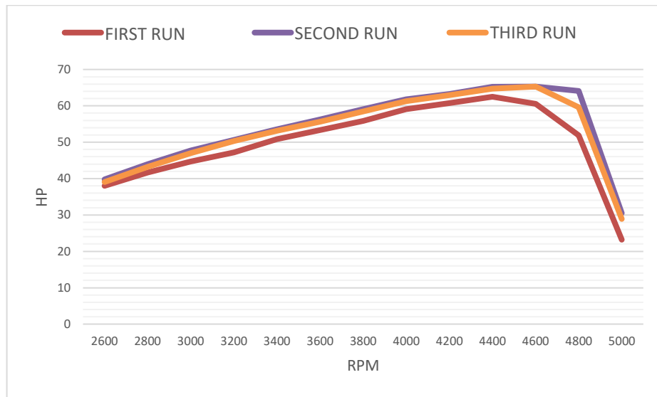
Fig. 7. Vehicle power with the cylinder head modification during three runs
