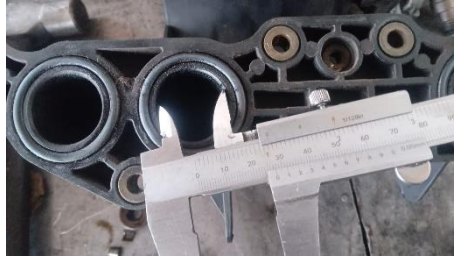
Fig. 3. Measurement of the intake manifold nozzle diameter
