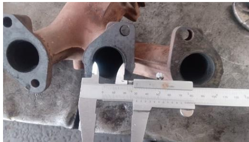
Fig. 2. Measurement of the exhaust manifold nozzle diameter
